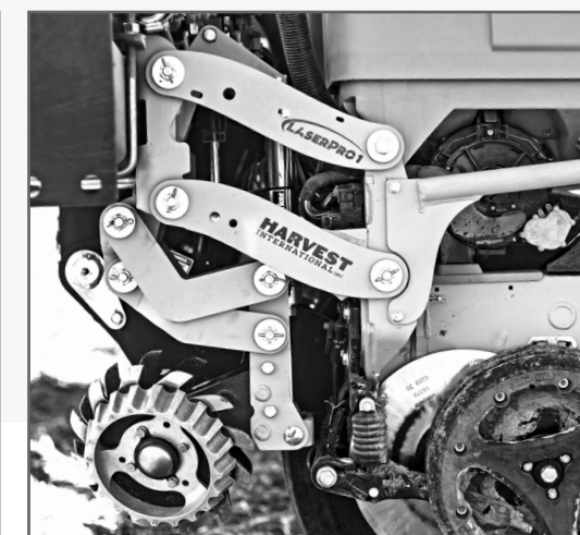
LASERPRO1 + integrated LASERSWEEP™ row cleaner Integrated X-plate mount with no in-field row unit interference
